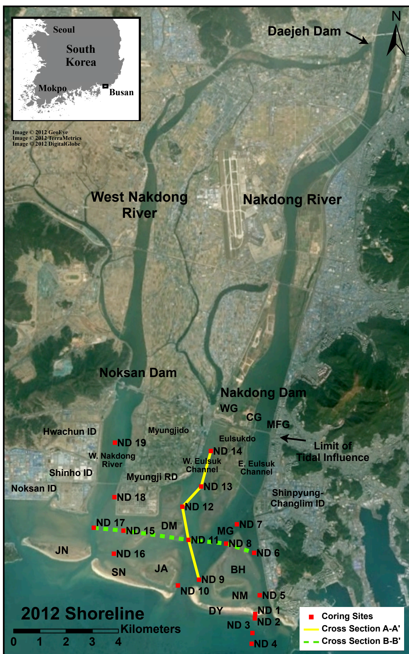
Fig. 1) Detailed study area map showing core sampling locations and cross sections. Noksan, Nakdong, and Daejeon Dam locations, channel names, barrier islands, and industrial (ID) and residential districts (RD) are indicated (WG=Western gate, CG=Control gate, MFG=Main floodgate, JN=Injudo, DM=Daemadaeung, JA=Jangjado, BY=Bakhabdeung, SN=Sinjado, DY=Dooyeung, NM=Namutitdeung, and MG=Maenggeummeorideung).
